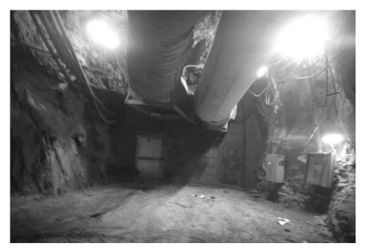
Picture 6. A station with fresh air with two air tube suppliers
